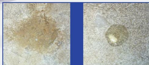
The stone surfaces above were affected by mineral seal oil. On the left (untreated side), the oil has left an immediate stain, while the oil on the right side (treated with SURFACE BARRIER™) has “beaded-up” and can be removed easily without staining the stone.
